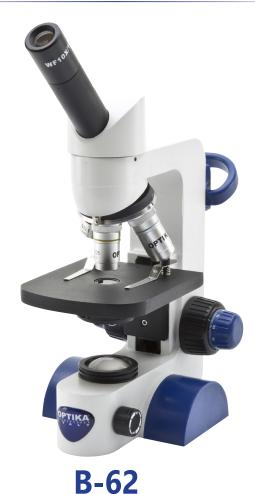
Cordless, modern monocular microscope ideal for students and mainly primary schools with achromatic lenses (400x), FN 18 eyepiece, finite optical system, coaxial focusing, StagErase™ eraseable fixed stage and 1 W LED illumination with rechargeable batteries. Slim and easy to carry, it is equipped with arm/wrist rest support to reduce the fatigue during use and long lasting LED illumination to provide over 20 years of use
