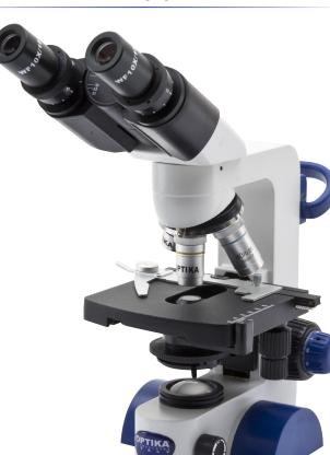
Cordless, modern binocular microscope ideal for students and mainly primary schools with achromatic lenses (400x), FN 18 eyepieces, finite optical system, coaxial focusing, StagErase<sup>™</sup> eraseable mechanical stage, Abbe condenser and 1 W LED illumination with rechargeable batteries. Slim and easy to carry, it is equipped with arm/wrist rest support to reduce the fatigue during use and long lasting LED illumination to provide over 20 years of use
