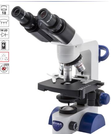
Cordless, modern binocular microscope ideal for students and mainly primary schools with achromatic lenses (1000x), FN 18 eyepieces, finite optical system, coaxial focusing, StagErase<sup>™</sup> eraseable mechanical stage, Abbe condenser and 1 W LED illumination with rechargeable batteries. Slim and easy to carry, it is equipped with arm/wrist rest support to reduce the fatigue during use and long lasting LED illumination to provide over 20 years of use
