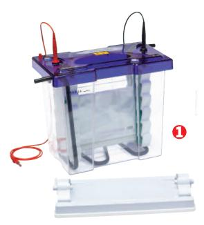
Each Modular System comprises the Gel Chamber, PAGE Internal Running Module, Casting Base and various accessories. Through the addition of further modules, the packages flexibility is increased to allow Western blotting and Capillary IEF.
