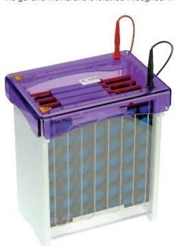
maintained. These units are compatible with magnetic stirrers to aid heat dispersal and prevent pH drifts in the buffer due to incomplete buffer mixing. Each system includes a cooling pack to further enhance transfer efficiency by removing excess heat. This also saves on buffer for added economy.
