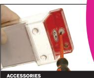
Cassette-style electrodes - difficult to break, but inexpensive and easy to change - composed of 99.99% corrosion-resistant, pure platinum.
