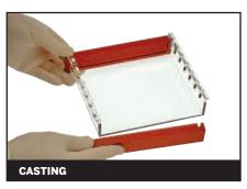
'Plug-and-Go' casting - moulded casting dams clip easily onto the ends of the gel tray for rapid external casting, allowing the multiSUB™ unit to remain in use for gel running. Casting is as simple as 1, 2, 3... place one dam onto the lab bench facing upwards and insert the tray into the groove in the dam and repeat with the second dam at the other end. The tray is now sealed and may be placed on flat bench space or gel levelling table in readiness for leak proof gel-casting.
