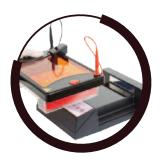
place the gel tank and agarose gel onto the base station
