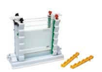
**External Casting Upstand is** basically a standard internal module but without Platinum wire
