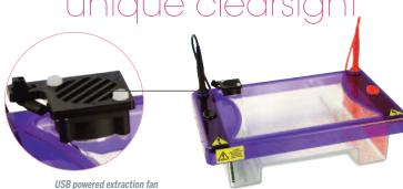
ClearSight lids solve the condensation build-up problem and so provide a perfectly clear view of the gel and the dye lane progression during the run. This is achieved using a  $\ensuremath{\mathsf{USB}}$ powered extraction fan within the lid. ClearSight lids are available as components of complete systems or as upgrades.
