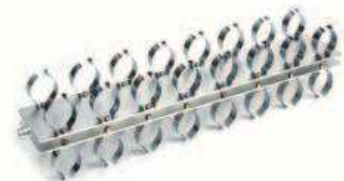
VM80-C Tube Holder Frame: 50ml Sharp Bottom Tube x 16
