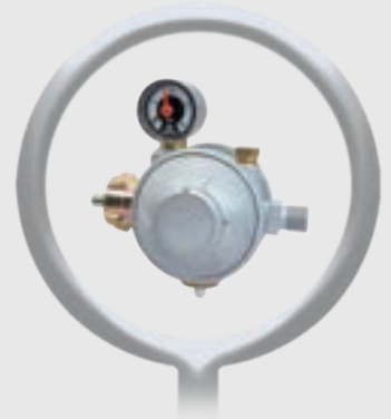
DVGW low pressure regulator DIN 4811-4, for household liquid gas installation, with overpress.-, temperature- fuse & manometer, for gas bottles up to 14 kg Art.-No. 6.000.150
