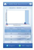
Software Intelligence: Automatically generates standard curves and directly outputs concentration of unknown samples.
